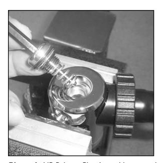
**Photo I** HP Balance Plug Assembly removal Flathead-VI or DS-IV (DS-IV shown)
