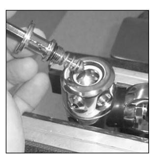
**Photo 2** Turret Bolt Assembly removal (50D only)
