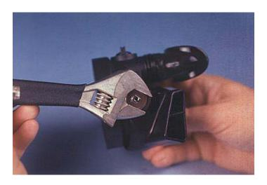
Tighten the Adjustment knob tube cap RG1417 with a flat jawed adjustable wrench
