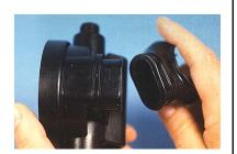
24) Use a small flat tipped screwdriver CAREFULLY pry the exhaust tee loose by using the small spaces provided under the Inlet and Adjustment tube ports
