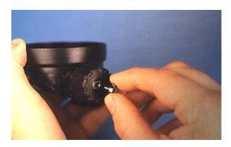
18) Using the eraser of a #2 pencil compress the piston to the point where the washers are exposed.
