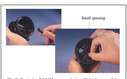
The Deflect tube RG1422 can now be installed take note of the orientation. Small opening faces out The larger orifice faces the mouthpiece tube.
