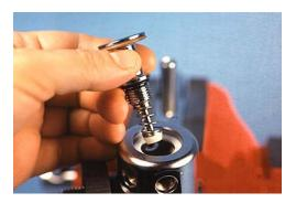
21) Tighten with a 6mm hex wrench ( Be careful not to crimp "O" ring )
