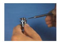
4) Using a 3/4 inch wrench remove the Inlet Nipple remove the "O" ring from the Inlet Nipple
