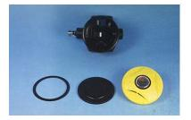
6) Remove the retainer ring and diaphragm
