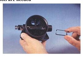
Note: If the Orifice was not screwed into the inlet nipple as previously mentioned the Lever Arm will be improperly installed
