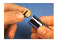
8) Place the Din hand wheel over the Din connector ( the threads face away from the first stage block)
