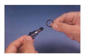
Remove the "o" ring RG1404 from the Adjustment tube assembly
