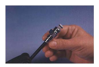
After loosening the orifice completely use a 6mm Allen key to push the orifice The Orifice will be returned to Dive Rite The rebuild kit is supplied with a new Orifice
