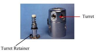
14 ) Remove the high pressure valve and spring
