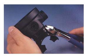
Remove Mouthpiece RG1273 by cutting Nylon Tie
