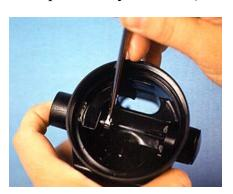
10) Using a # 2 pencil compress the the piston to the point that the spacing washers are exposed
