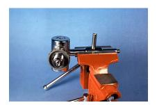
3) Using a 6mm Hex wrench loosen the adjustment screw enough to lessen the spring tension
