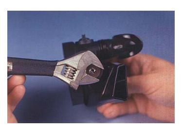
Loosen the Adjustment knob tube cap with a flat jawed adjustable wrench
