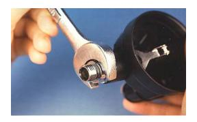
3) Using a 3/4 inch wrench loosen and the remove the Inlet Nipple
