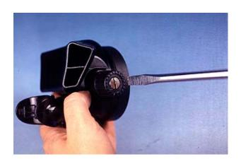
Using a Flat tipped Screwdriver loosen and remove Knob Screw RG1419
