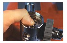
24) Install the Diaphragm (Make certain that the diaphragm is seated below the threads and is in contact with the seating surface
