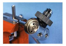
22) Turn the first stage over so the balance chamber is facing up
