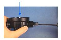
13) Using a flat head screwdriver turn the inlet valve until the lever arm is just slightly above the second stage cover threads
