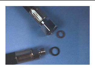
29) Lubricate and install "O" rings and on the low pressure hose. Install the hose into a LOW pressure port on the RG1200 First stage
