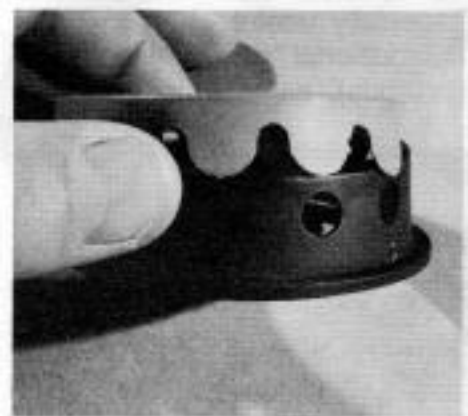
12-port, large-area exhaust valve ring.
