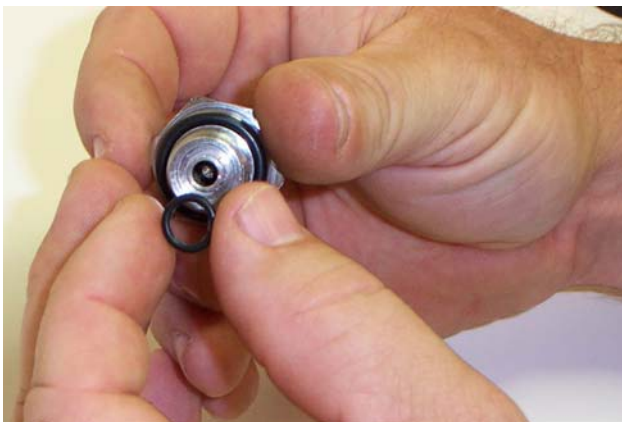
Figure 4-18 This O-ring must be installed in the bottom
