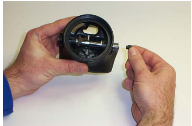
Figure 6-11. The Spacer is installed after the Spring.
