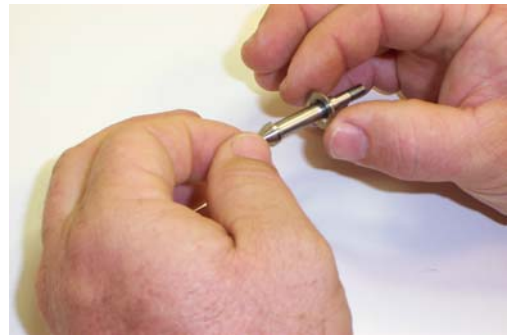
Figure 4-2 Install the Small Packing Disk on the Poppet.
