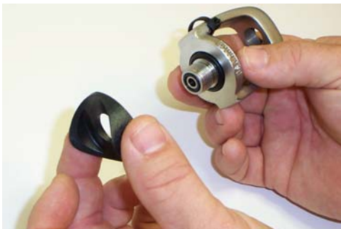
Figure 3-8 Separate the Saddle from the Yoke
