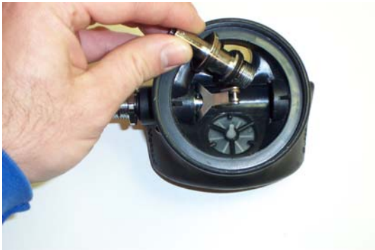
Figure 6-8. The Adjustment Sleeve must be angled into the Regulator Can.
