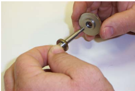
Figure 4-5 Install the Large Packing Disc.
