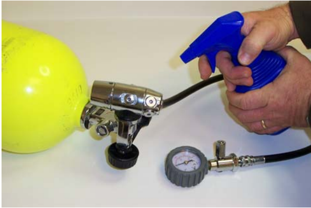
Figure 4-21 Leak testing the First Stage.
