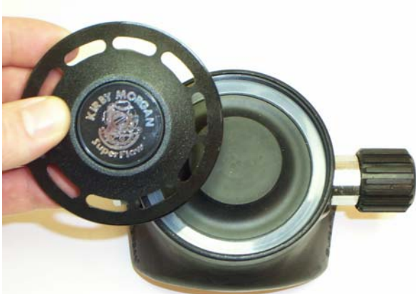
Figure 5-3 Remove the Second Stage Cover.
