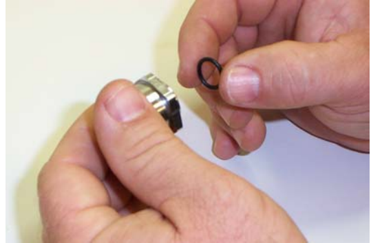
Figure 4-15 Make sure the O-ring has been installed underneath the Sintered Filter.
