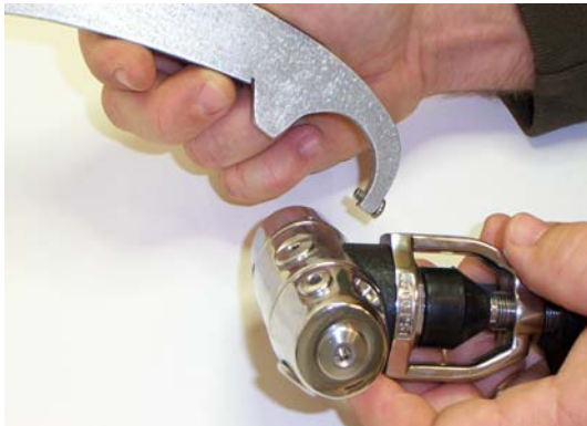
Figure 4-13 The spanner wrench is used to tighten the Cap.
