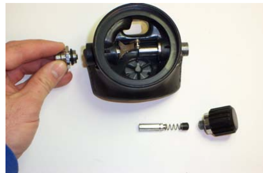
Figure 5-6 Remove the Inlet Nipple.
