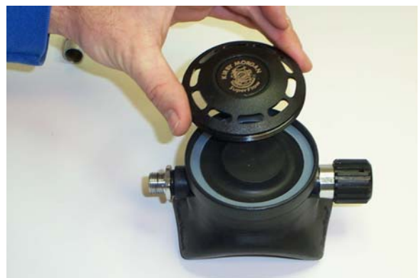
Figure 6-17. Install the Regulator Cover.
