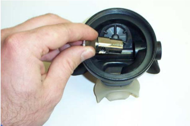
Figure 5-8. Removing the Inlet Valve/Roller Lever Assembly.
