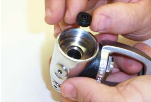
Figure 4-12 Insert the new Seat (23) with new O-ring (22) in the First Stage Body with the cone shaped end facing toward you when looking into the Large Bore Port.
