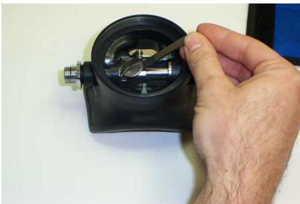
Figure 6-18. Insert the adjustment wrench under the legs of the Lever prior to bending the Lever down.
