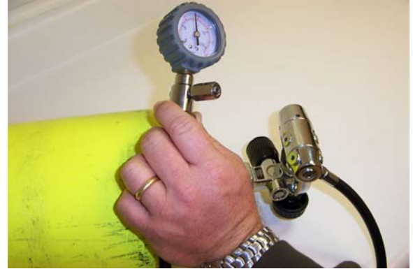
Figure 4-20 Testing the First Stage Pressure.
