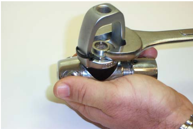
Figure 4-19 Tighten the Yoke Retainer.
