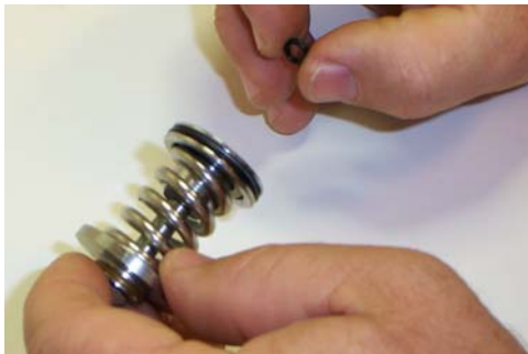
Figure 4-9 Place O-ring in the external Piston recess
