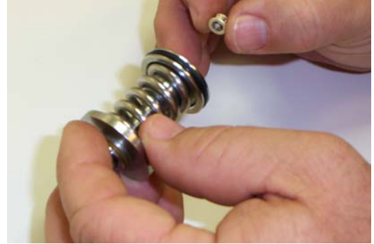
Figure 4-11 Thread the Nut onto the Poppet
