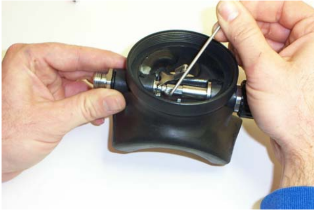
Figure 6-14. Minor adjustments are more easily done using the jewelers screw driver or large sewing needle.
