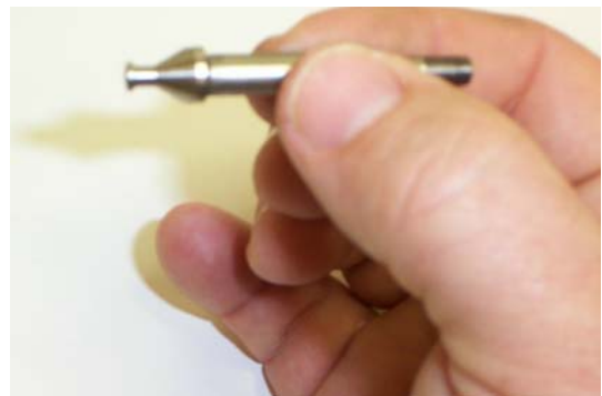
Figure 3-6 Inspect the Poppet Head for nicks. It should have a smooth, shiny finish.
