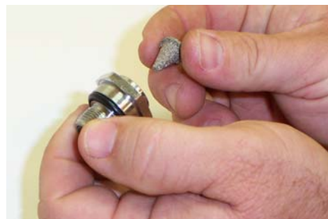
Figure 4-16 Install the Sintered Filter.
