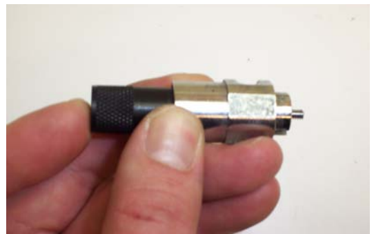
Figure 6-3. Compress the Spring with the Castle Wrench.
