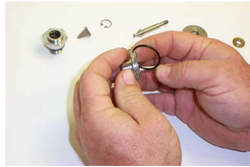
Figure 4-1 Install all of the O-rings except #10, 11, and 19
