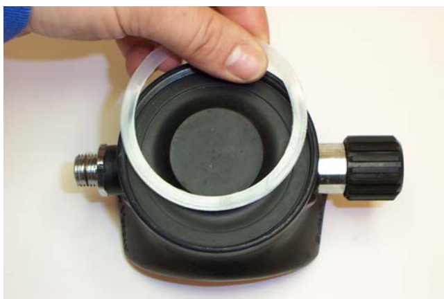
Figure 5-4 Remove the Diaphragm Washer.
