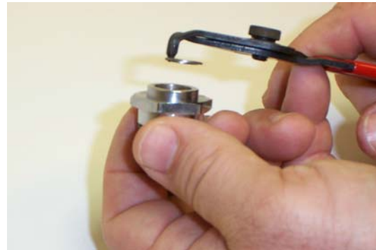
Figure 3-9 Remove the Circlip.
