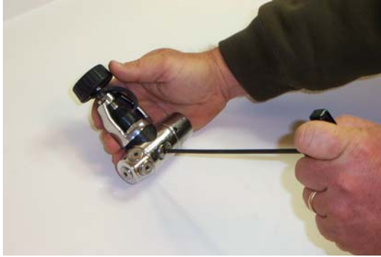
Figure 3-3 Removing High Pressure Plugs
