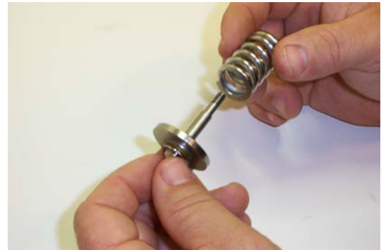
Figure 4-7. Slide the Spring onto the Poppet.
