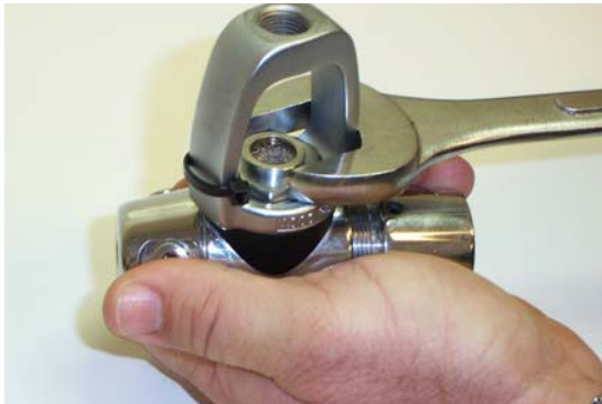
Figure 3-7 Loosen the Yoke Retainer.
