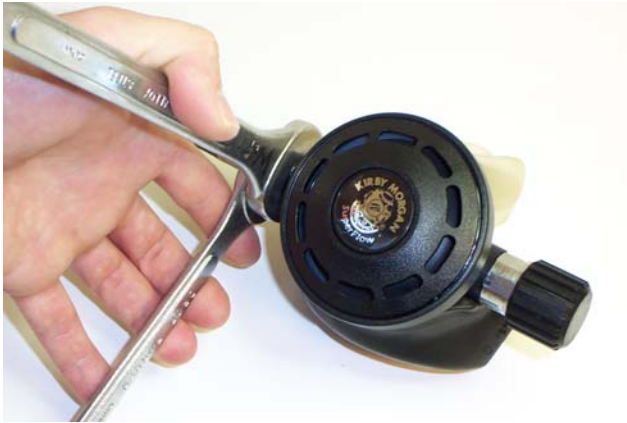
Figure 5-2. Remove the Low Pressure Hose.
