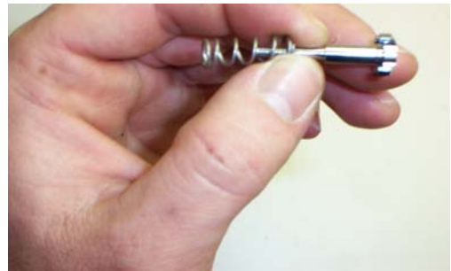
Figure 6-1. Install Inlet Valve on Spring.
