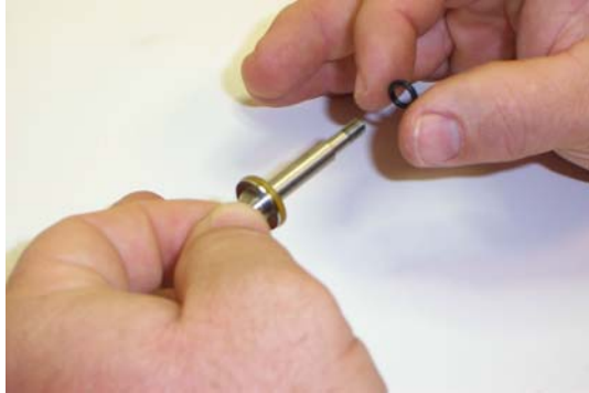
Figure 4-4 Install the O-ring on the Poppet.
