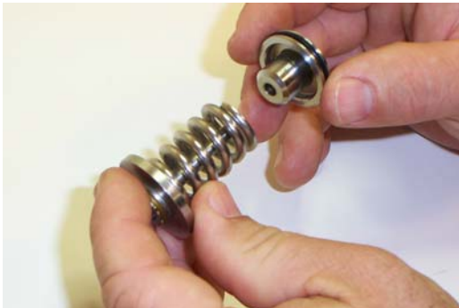
Figure 4-8 Install the Piston Head.
