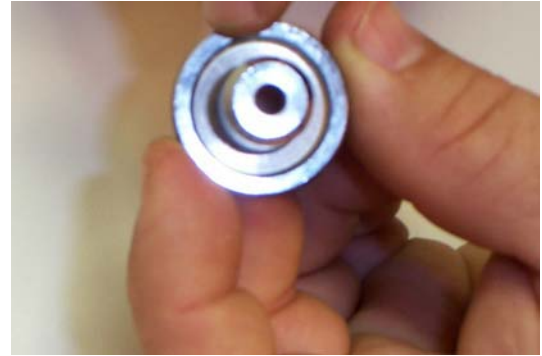
Figure 4-6 The Shims sit in the recess in the Piston Head.
