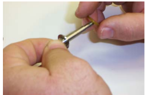
Figure 4-3 Install the urethane O-ring (11)
