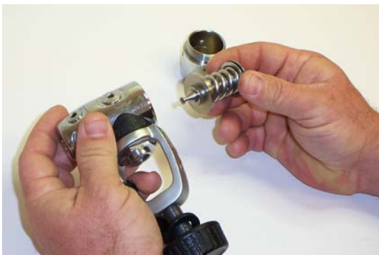
Figure 3-4 Removing the Piston/Spring Assembly from the First Stage Body
