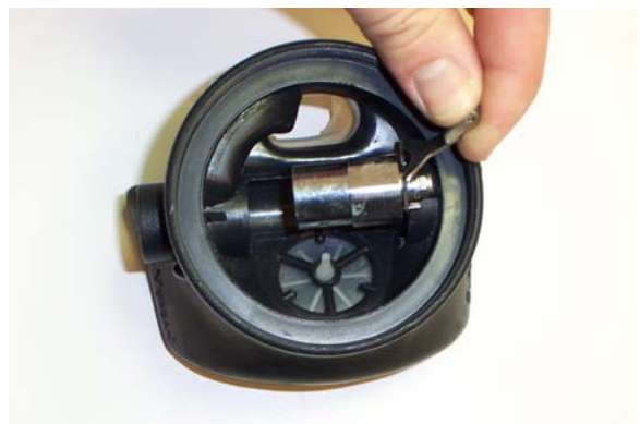
Figure 6-7. Installing the Roller Lever Assembly.
