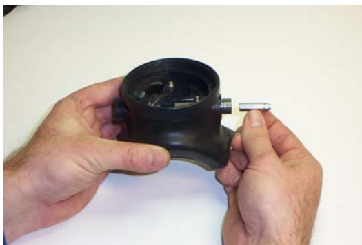
Figure 6-9. The machined end of the Piston faces the outside of the Regulator.
