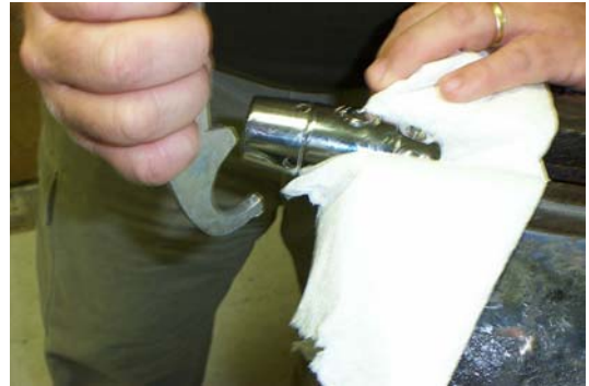
Figure 3-2. Placement of the first stage in a vise
