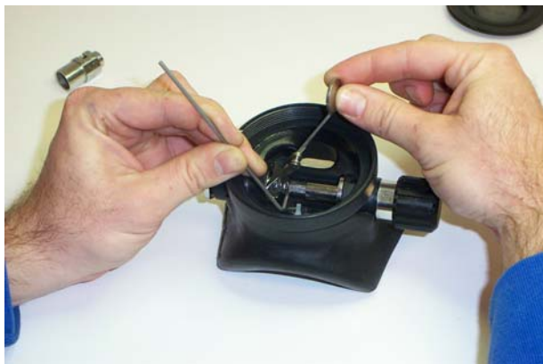
Figure 6-16. Use the Inlet Holder and wrench together to adjust the Regulator.
