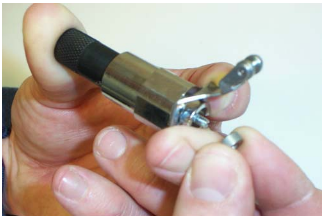
Figure 6-4. Place the Spacer on the threaded end of the Inlet Valve.
