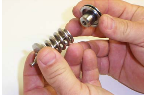
Figure 3-5 Remove the piston head from the poppet.
