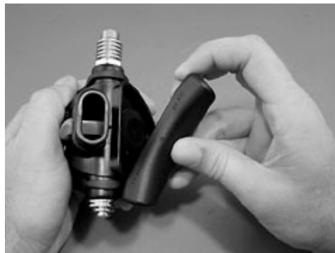
Fig. 2 – Removal of Exhaust Tee
