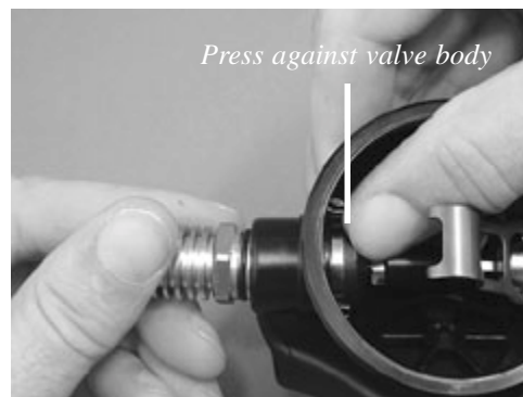
Fig. 22 – Install Inlet Fitting
