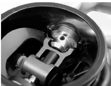
Fig. 19 – Installing Lever Assembly
