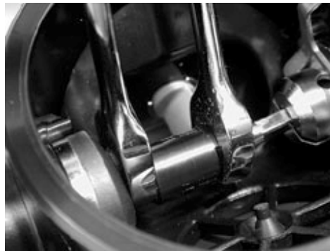
Fig. 21 – Tightening Connecting Nut to Sheath
