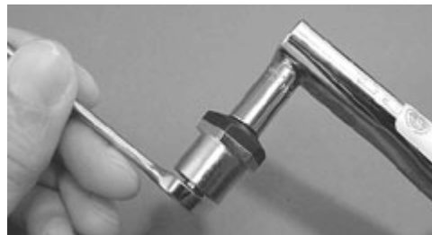
Fig. 17 – Torque Nut to Poppet
