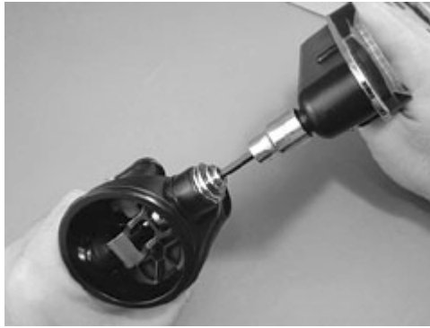
Fig. 25 – Torque Plug to xx Inch-Pounds
