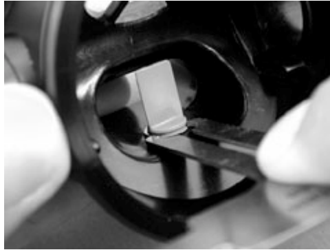
Fig. 8 – V.A.S. Circlip Removal
