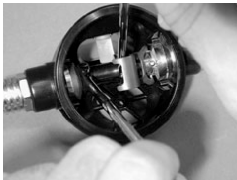
Fig. 5 – Loosen Connecting Nut and Sheath
