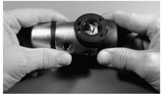
Fig. 6 – Removal of Saddle
