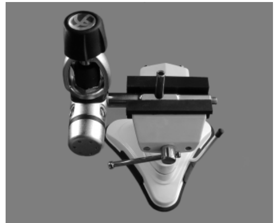
Fig. 1 – Recommended Vise Mounting
