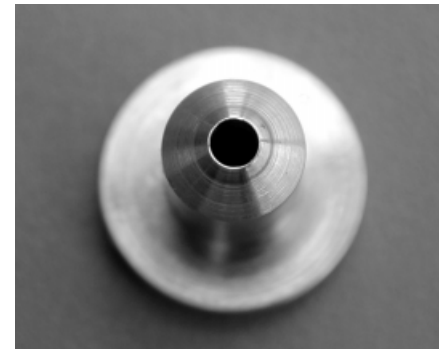
Fig. 12 – Inspection of Orifice
