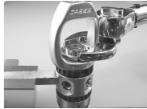
Figure 22. Torque inlet fitting
