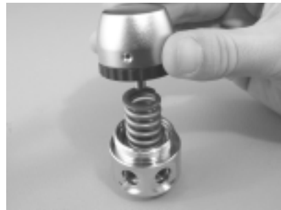
Figure 13. Install end cap
