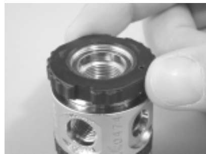
Figure 15. Install adjustment ring
