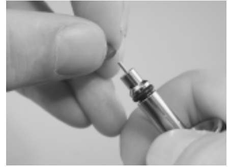
Figure 6. Push out HP seat
