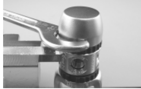
Figure 21. Tighten end cap
