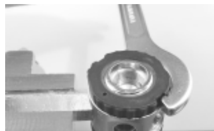
Figure 3. Remove adjustment ring
