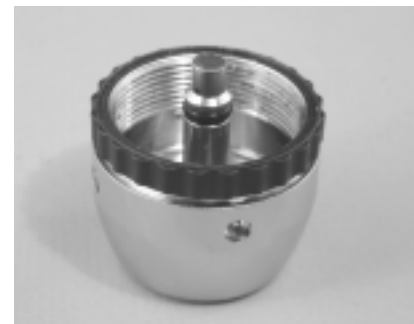
Figure 10. Press piston into end cap
