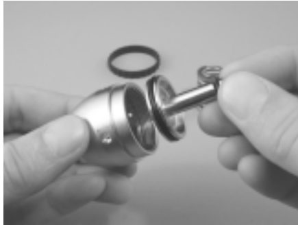
Figure 5. Remove piston from end cap
