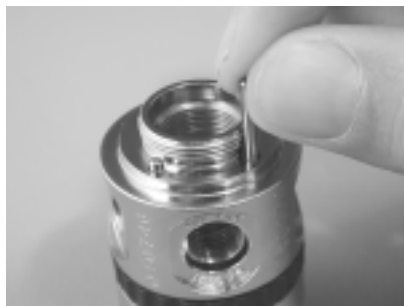
Figure 14. Install adjustment pins
