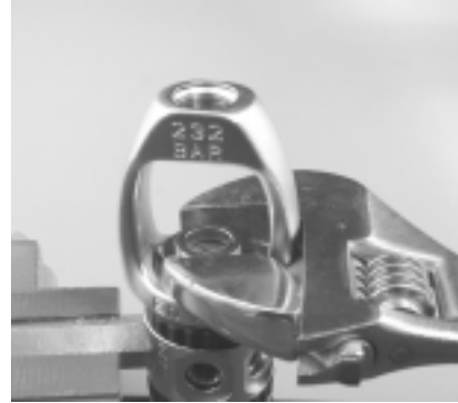
Figure 1. Mount first stage in vise and remove inlet fitting
