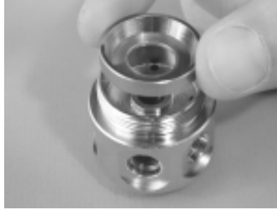
Figure 11. Install spring support
