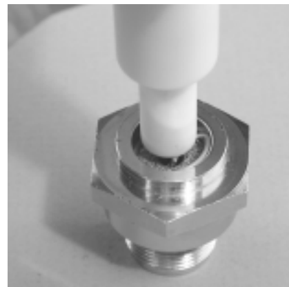
Figure 19. Compress clip to ensure it is securely in place
