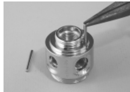
Figure 8. Remove adjustment springs
