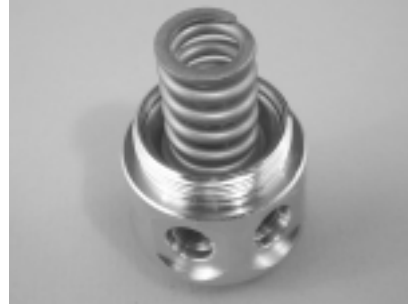
Figure 12. Install main spring
