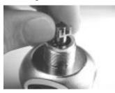
Figure 21. Install balance chamber into sleeve.
