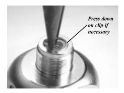
Figure 24. Install filter retaining clip
