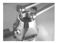
Figure 2. Remove spring retainer
