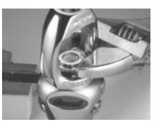
Figure 6. Remove yoke retainer
