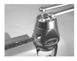
Figure 36. Tighten spring retainer with adjustable face spanner wrench until it stops
