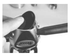
Figure 3. Remove diaphragm with a short blast of low pressure air
