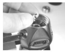
Figure 4. Remove the pin support
