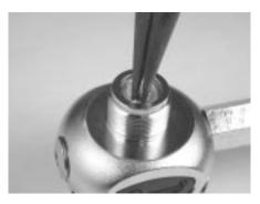
Figure 7. Remove filter retaining clip and filter
