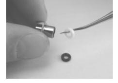
Figure 10. Remove O-ring and backup ring from balance chamber
