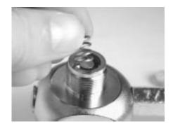
Figure 8. Remove balance chamber spring
