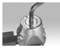
Figure 1. Mount first stage in vise and remove adjustment screw
