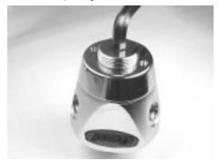
Figure 32. Screw in adjustment screw until flush with spring retainer
