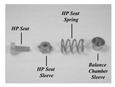
Figure 12. Separate parts
