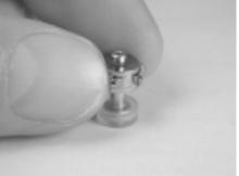
Figure 14. Install sleeve onto HP seat
