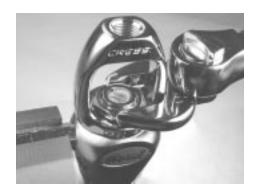
Figure 35. Tighten retainer to 20 footpounds
