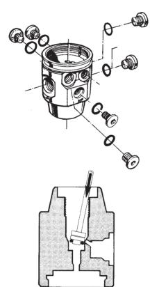
2. Screw in the blind screws in the LP- HP outlets. Use a 5 mm Allen wrench and tighten up by hand.
