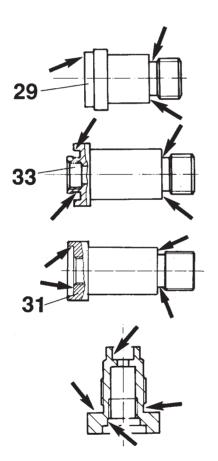
4. The connections (29,31 or 33). Check to make sure the sealing surfaces for the o-rings are undamaged.
