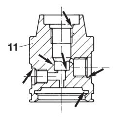
3. The valve housing (11). Check to make sure the threads and also the sealing surfaces for the o-rings are undamaged.
