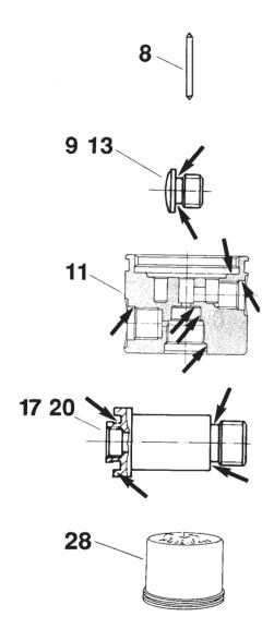
When servicing the regulator following parts should be replaced:
