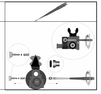
Disassemble the air barrel and all of its components.
