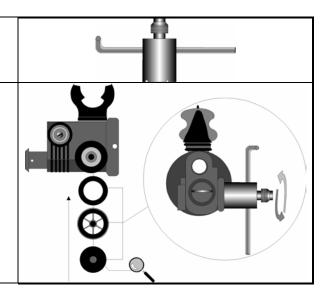
Inspect and lubricate the inflator mechanism cover o'ring.
