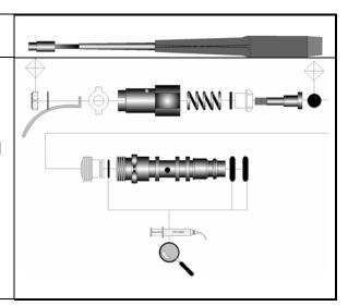
Insert the air barrel assembly into the Air 2 body.
