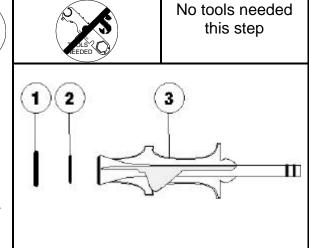
Inspect the o'ring (01.050.160) from the G250 air barrel. Replace only if there is damage or if there is a loss of flexibility. Lubricate to static o'ring specifications.
