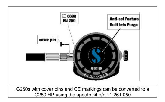
*Procedure for Converting a G250 into a G250 HP* Note: This procedure is only applicable to G250s fitting the description above.
